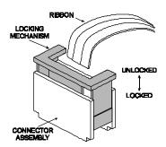
Figure 3-6. Ribbon Connector Locking Mechanism.
